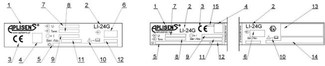
Figure 3. Examples of LI-24G transmitter nameplates in standard and Exi version
