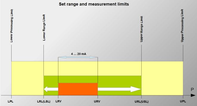
Figure 1. Set range and measurement limits
