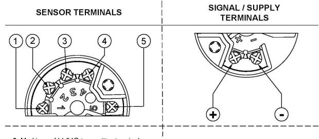
Figure 9. Markings of LI-24G transmitter terminals
