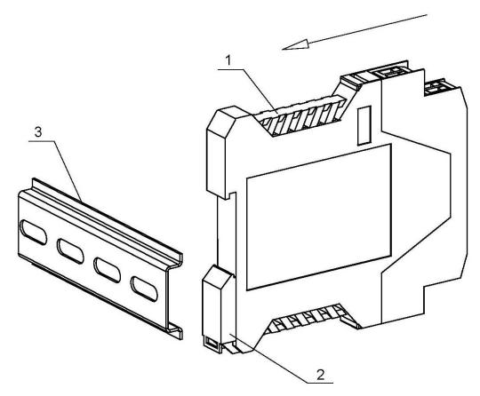
Figure 5. LI-24L transmitter installation on a DIN rail
