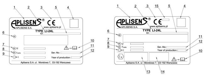
Figure 4. Examples of LI-24L transmitter nameplates in standard and Exi version
