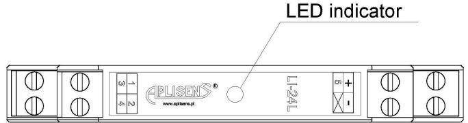
Figure 15. LED indicator on the LI-24L transmitter
