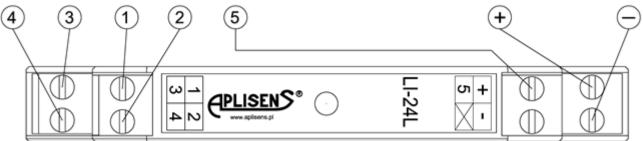
Figure 8. Markings of LI-24L transmitter terminals
