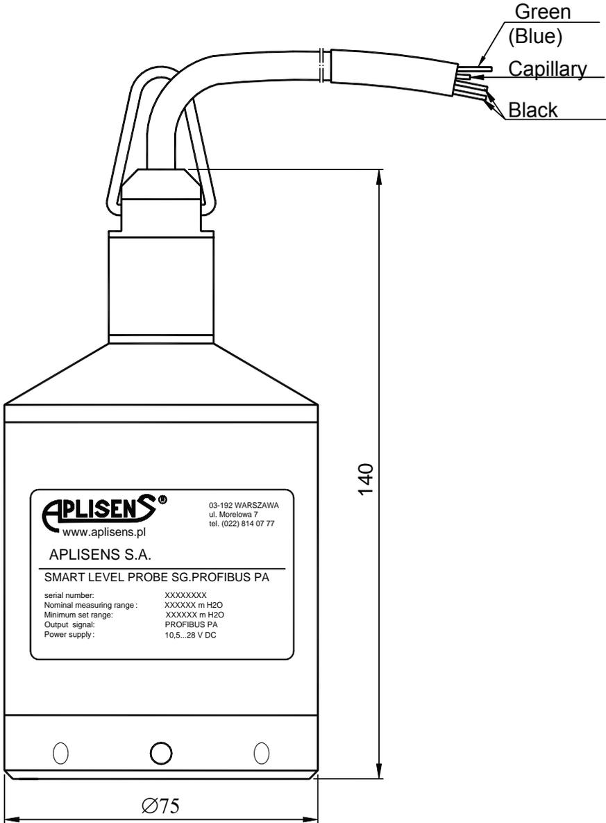
Fig.16. Smart level probe SG.Profibus PA - dimensions.
