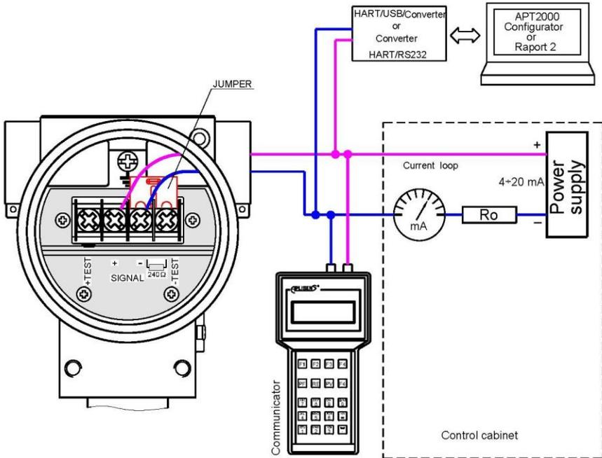
**Fig.2a.** The link of transmitter and communicator or converter to current line by the switch box (in case of the resistance in current loop is higher than  $240\Omega$ ).
