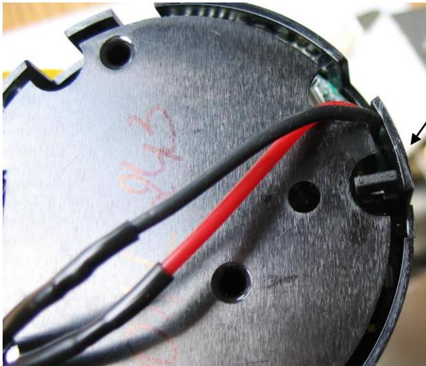
Jumper in radial position (as at photo) –back lighting off; jumper in circular position –back lighting on.
