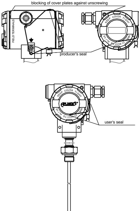
Fig 1c. APT-2000ALW in MID application. Sealed up transmitter.
