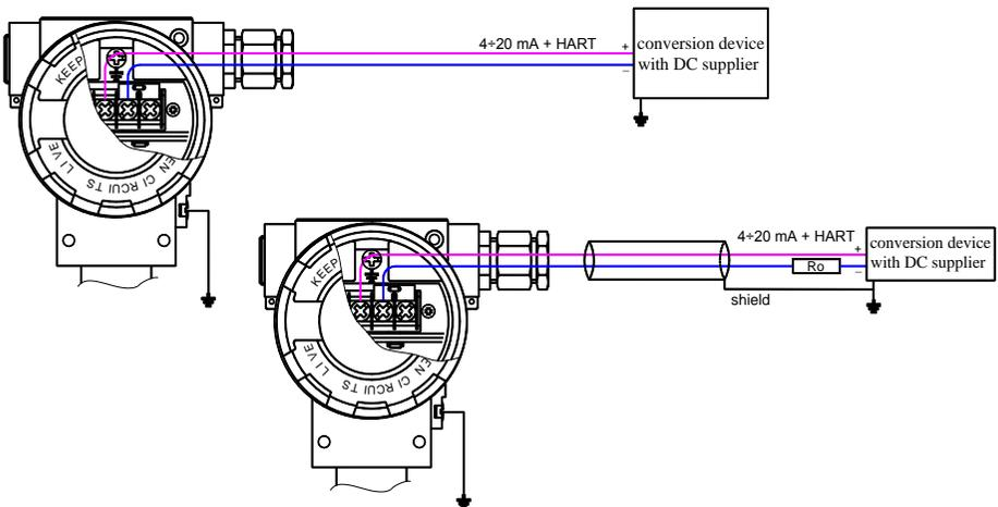
Fig. 1b. APT-2000ALW temperature transmitter for MID application.
