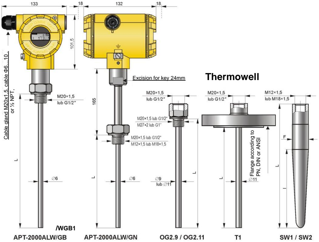
Fig.6. The types of shields of measuring insert.
