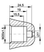
Fig.7b. Socket for M-type connector.
