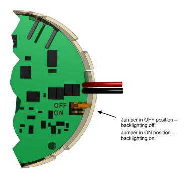
Figure 6b. Backlighting jumper view at transmitter electric board (unit display back side)
