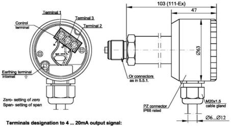
Terminal 1 - Supply "+" (plus) Terminal 2 - Supply "-" (minus) Terminal 3 - TEST SIGNAL
