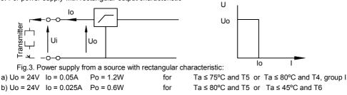
The supply of power from a source with a rectangular characteristic means that the voltage of the Ex power supply remains constant until current limitation activates.
