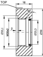
Fig.9c. Weldable fitting ring for CM30x2-type connector Sealing: teflon
