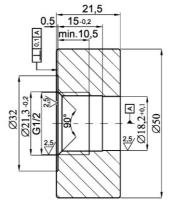
Fig.10d. Weldable fitting ring for use with transmitters with CG1/2 - type connector Material – 316Lss Order code Socket CG1/2
