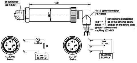
Wiring diagrams for transmitters with terminal PM12 (Not applicable to Ex version)
