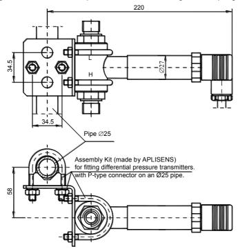
Figure 15. Example: how to install the PRE-28
