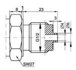
Fig.10a. G1/2-type connector with G1/2" thread
