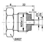
Fig.7a. M-type connector with M20x1.5 thread
