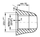
Fig.8b. Socket for P-type connector, (GP-type connector)
