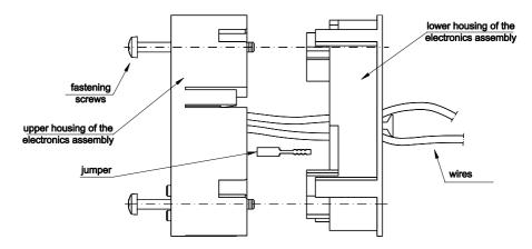
Figure 6a. View of disassembled display assembly
