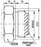
Fig.9a. CM30x2-type connector with flush diaphragm with M30x2 thread,
