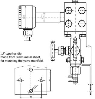
Figure 17. Example: how to install the PRE-28 transmitter with a valve manifold to a wall
