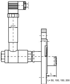
Figure 14. PRE-28 differential pressure transmitter with a single direct diaphragm seal
