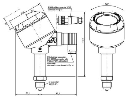
Figure 3. PCE-28 transmitter with ALW-type connector: dimensions and methods of connection
