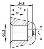
Fig.10b. Socket for use with transmitters with G1/2-type connector
