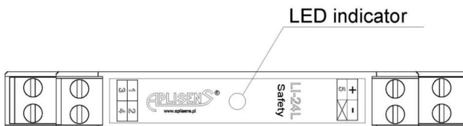
**Figure 1.** LED indicator in LI-24L Safety transmitter.
