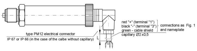
Figure 6. Connection of the transmitter with PM12 electrical connector
