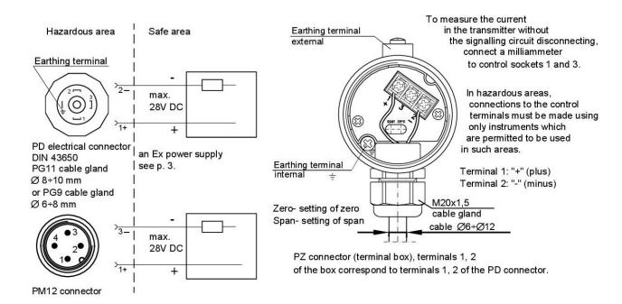
Figure 1. Connection of the transmitter with PD and PM12 electrical connectors
