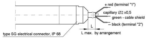
Figure 5. Connection of the transmitter with SG electrical connector
