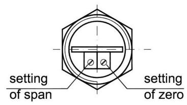
Figure 1. View of potentiometers of zero and span (PD, PK, PKD or PM12)
