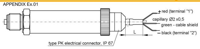
Figure 3. Connection of the transmitter with PK electrical connector
