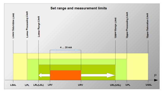
Figure 1. Set range and measurement limits
