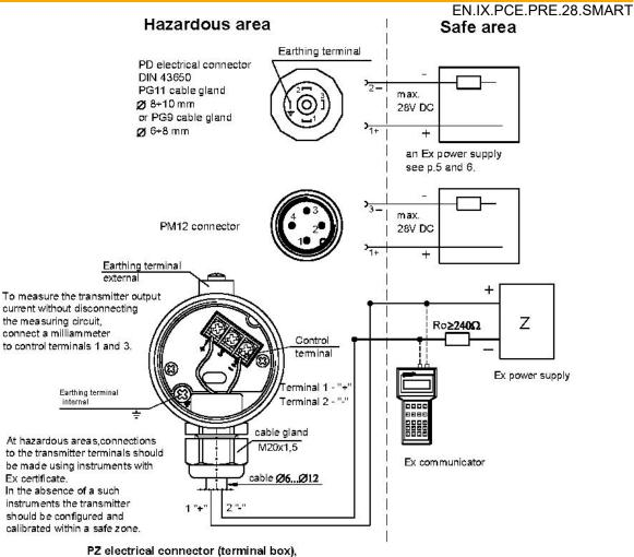
P2 electrical connector (terminal box), Terminals 1, 2 of the box correspond to terminals 1, 2 of the PD connector.
