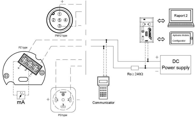
Figure 2. Electrical connection 4...20 mA of HART to transmitter in standard version
