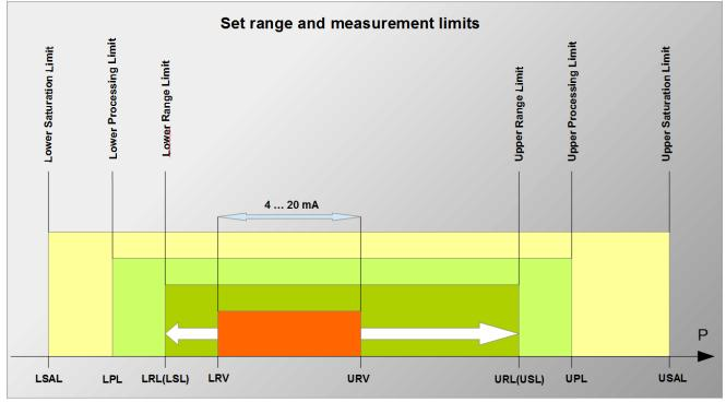
Figure 1. Set range and measurement limits
