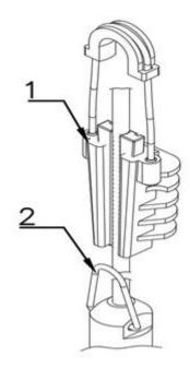
Figure 1 Mounting brackets for probes
