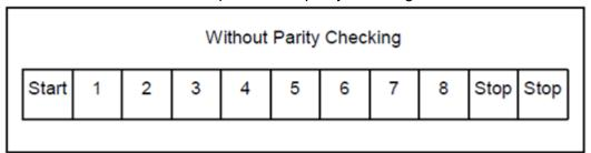
Bit sequence without parity checking.
