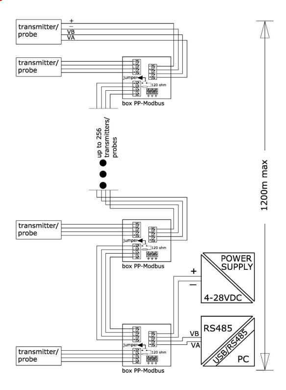
Figure 3 Connection in Modbus network
