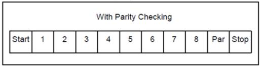
Bit sequence with parity checking.
