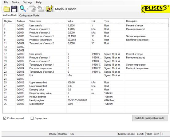
Switch the transmitter from Modbus into configuration mode working with Hart communication protocol.
