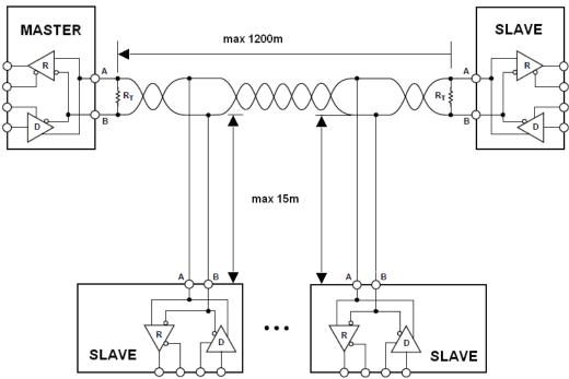
Figure 4 Example of Modbus network configuration
