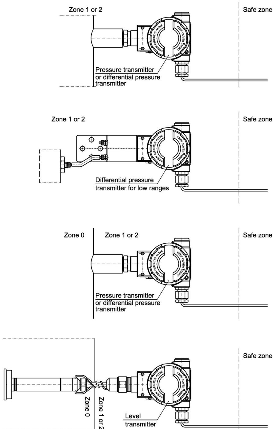
**Figure 2.** Transmitter installation in potentially explosive areas.
