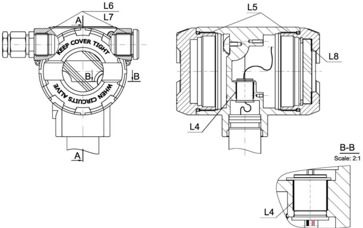
Figure 8. Flameproof joints of enclosure.
