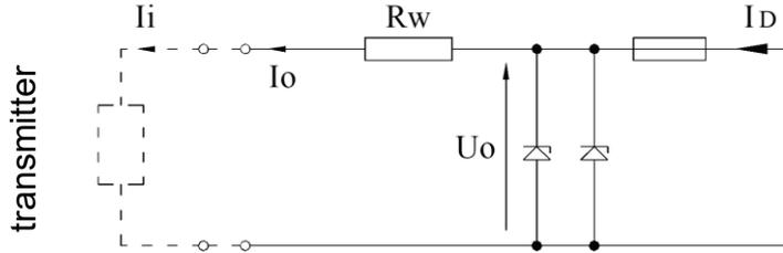
Figure 3. Principle of power supply from a linear source.
