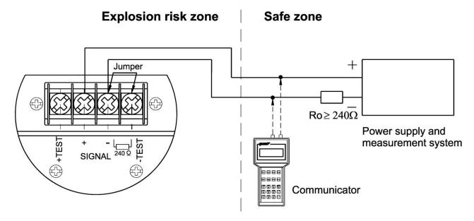
Figure 6. Connecting Exd transmitters and probes
