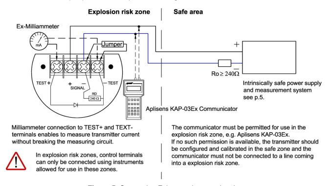
Figure 5. Connecting Exi transmitters and probes
