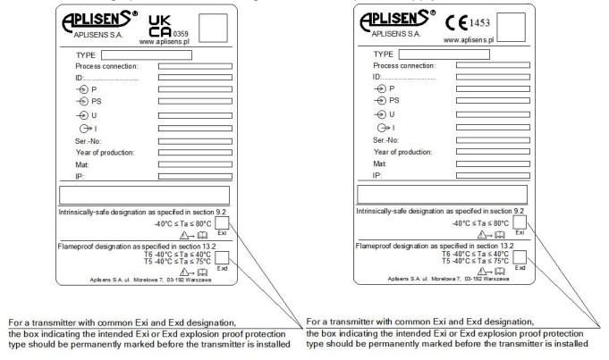
Figure 1. Sample transmitter nameplate with common Exi and Exd designation
