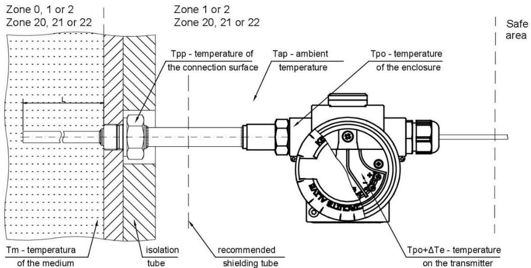
Figure 1. 8. Determining the working temperature of the transmitter.
