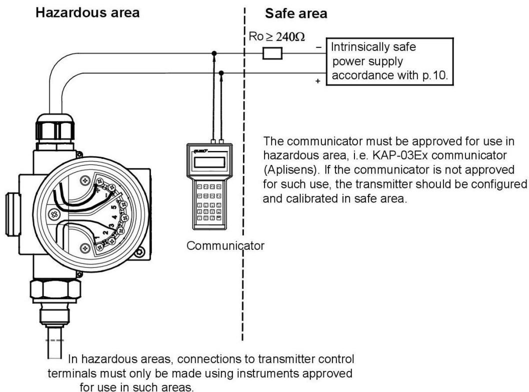
**Figure 1. 9.** Connection of the transmitter in Exi version.
