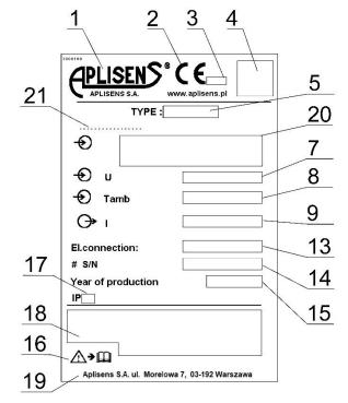
Figure 1.2. Example of a transmitter nameplate for use with an independent remote sensor.
