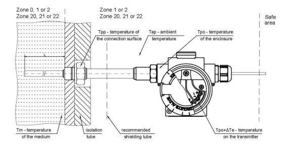
Figure 1.8. Determination of the temperature of transmitter.
