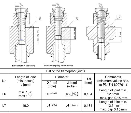
Figure 2. 10. The flameproof joints of the temperature sensors.
