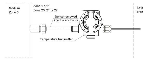
Figure 1. 4. LI-24ALW/C temperature transmitter with a sensor screwed into the enclosure.
