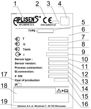
Figure 2. 1. An example of a nameplate for a transmitter with a direct sensor.
