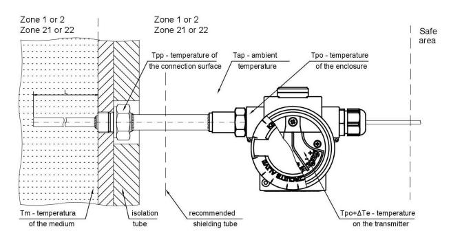
Figure 2. 6. Determination of the temperature of transmitter with sensor screwed into the enclosure.
