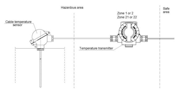
Figure 2. 3. LI-24ALW temperature transmitter with a cable temperature sensor.
