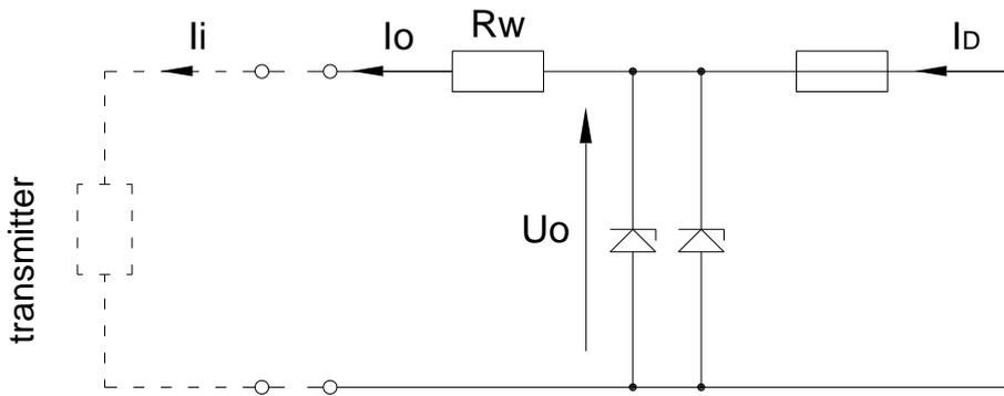
**Figure 14.** Linear power supply configuration
