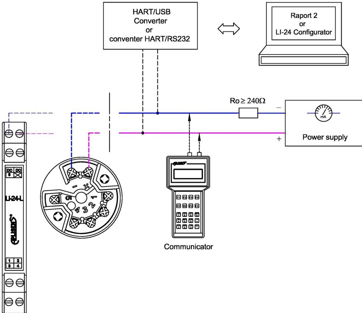
**Figure 10.** Electrical connection the transmitter in the safe areas
