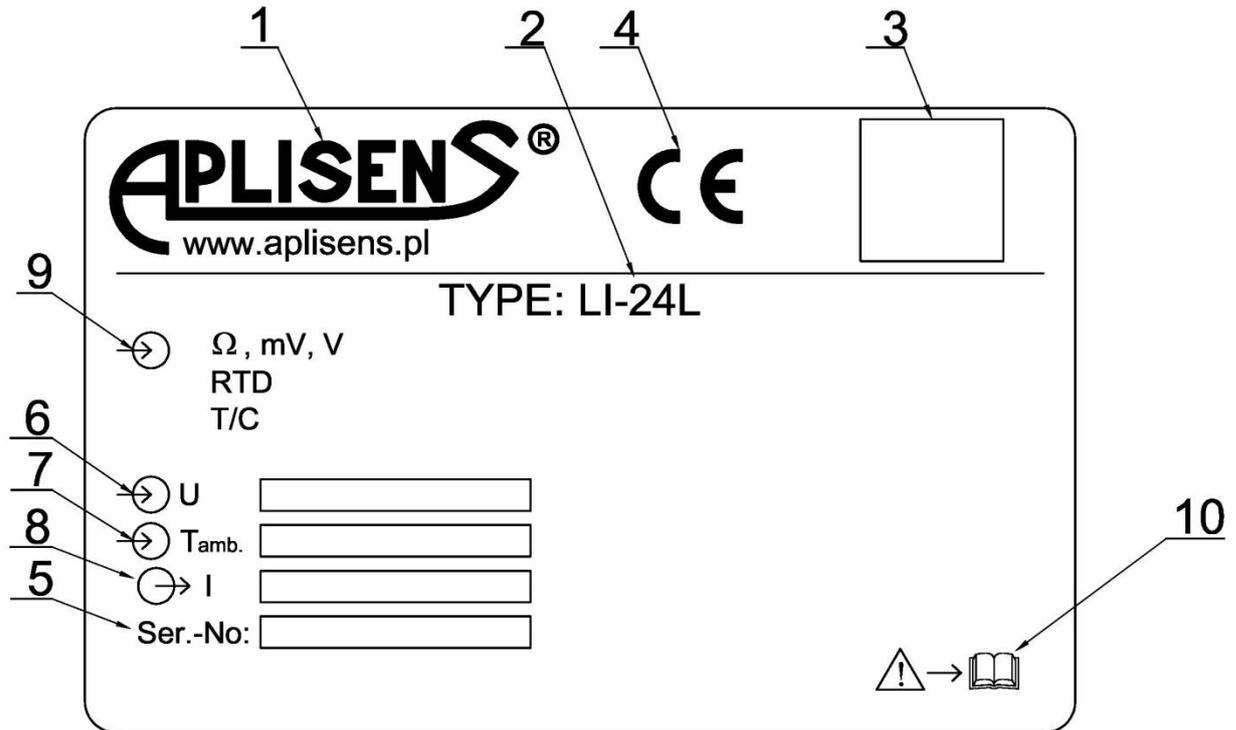
Figure 4. Example of the rating plate of LI-24L transmitter in normal version
