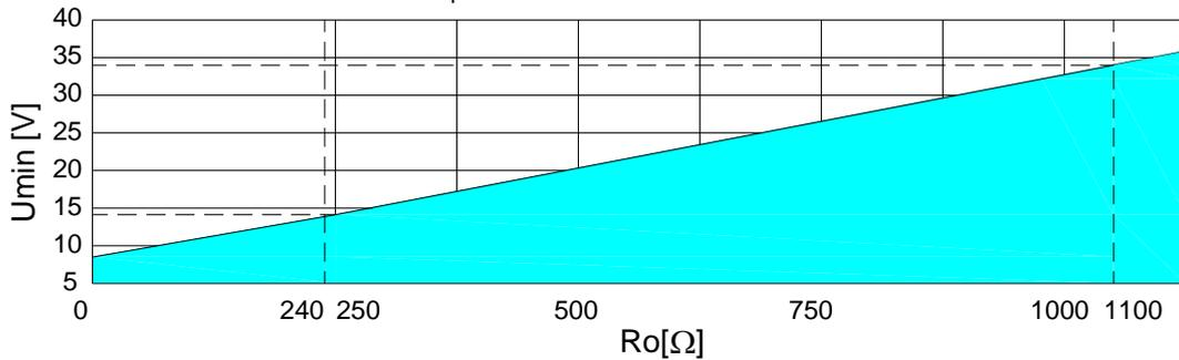
**Figure 13.** Correlation between supply voltage and resistance in the current loop
