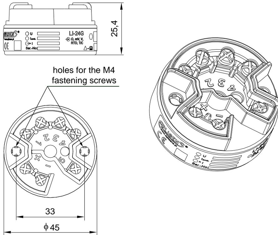
Figure 1. The LI-24G temperature transmitter. Dimensions
