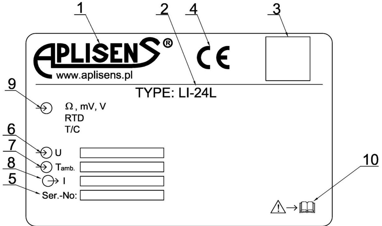
Figure 4. Example of the rating plate of LI-24L transmitter in normal version
