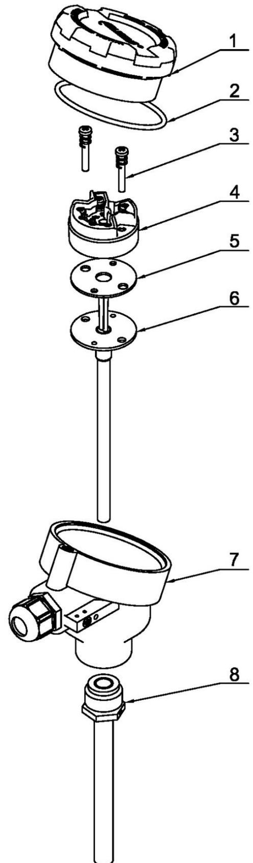
**Figure 6.** Mounting the LI-24G transmitter in the exemplary Aplisens connection head
