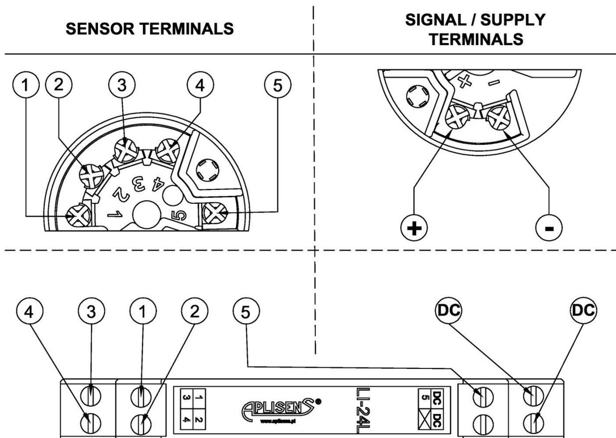
**Figure 8.** Designation of LI-24L and LI-24G transmitter terminals
