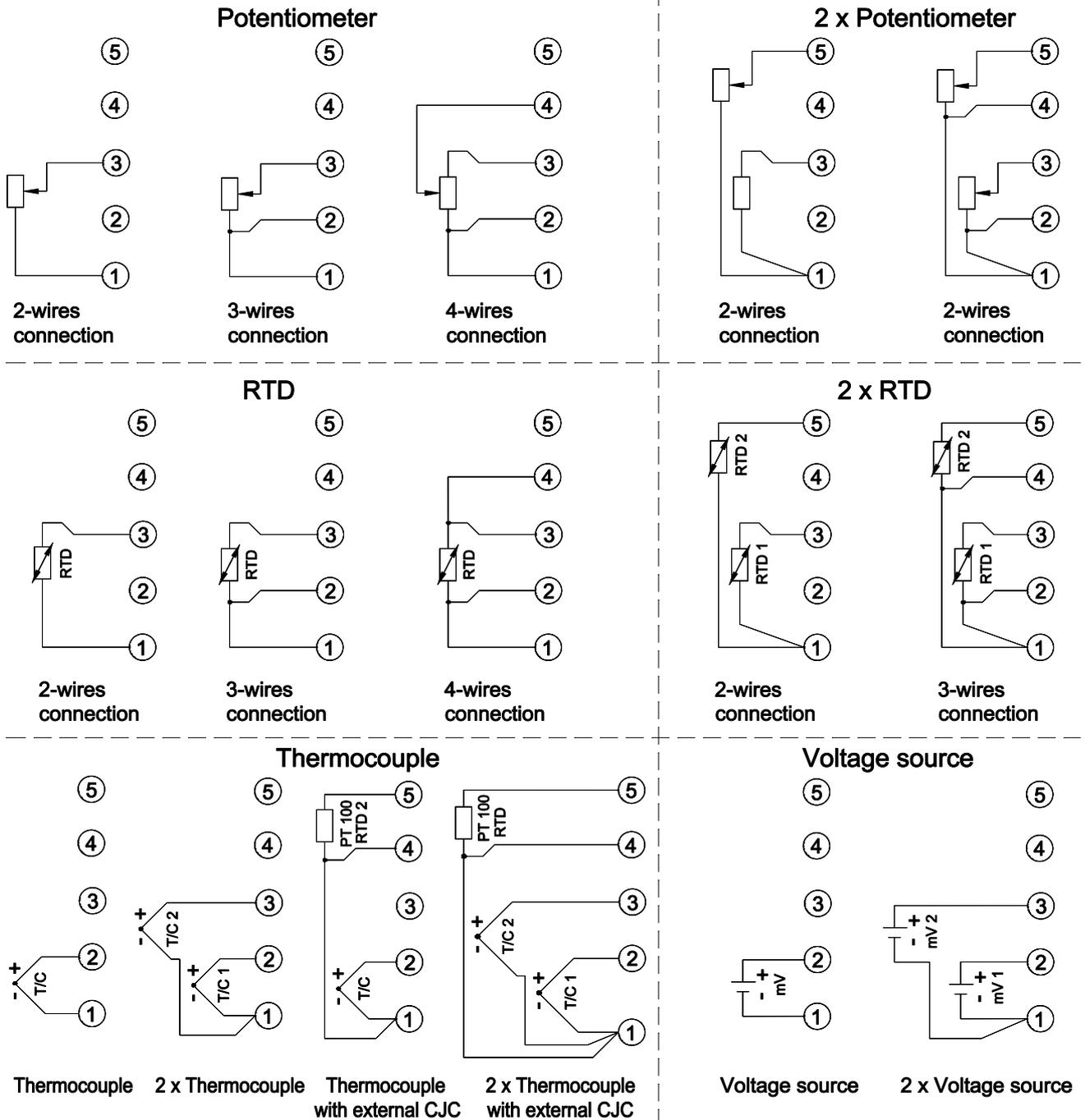
Figure 9. Possible ways of sensor connection
