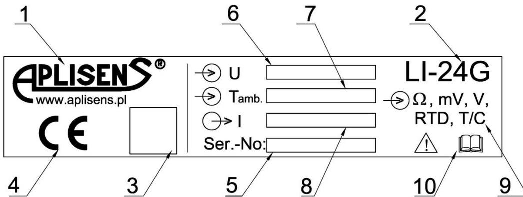
Example of the rating plate of LI-24G transmitter in normal version
