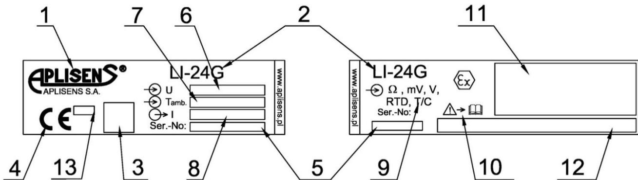
Example of the rating plate of LI-24G transmitter in Ex version
