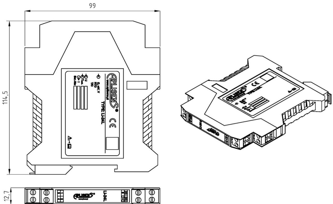
Figure 2. The LI-24L temperature transmitter. Dimensions
