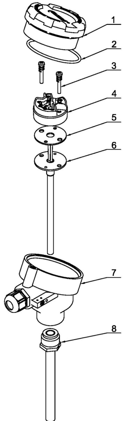
**Figure 6.** Mounting the LI-24G transmitter in the exemplary Aplisens connection head
