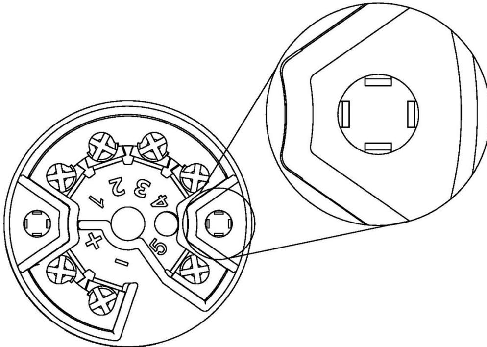
**Figure 7.** Protect against the fastening screws falling out
