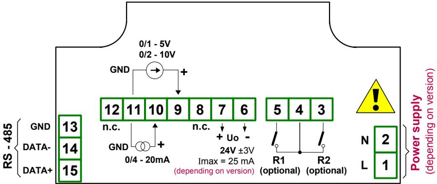
Figure 4.3. Terminals description (relay outputs)
