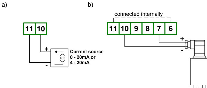
Figure 4.11. Connections of 2-wire sensor:
