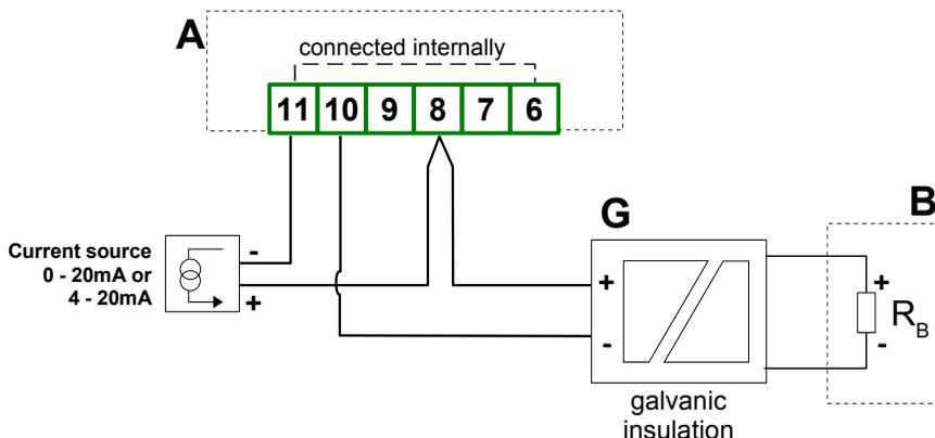
Figure 4.12. Serial connection of active 2-wire sensor with **PMS-620N** unit and other current measurement device (e.g. PLC controller).
